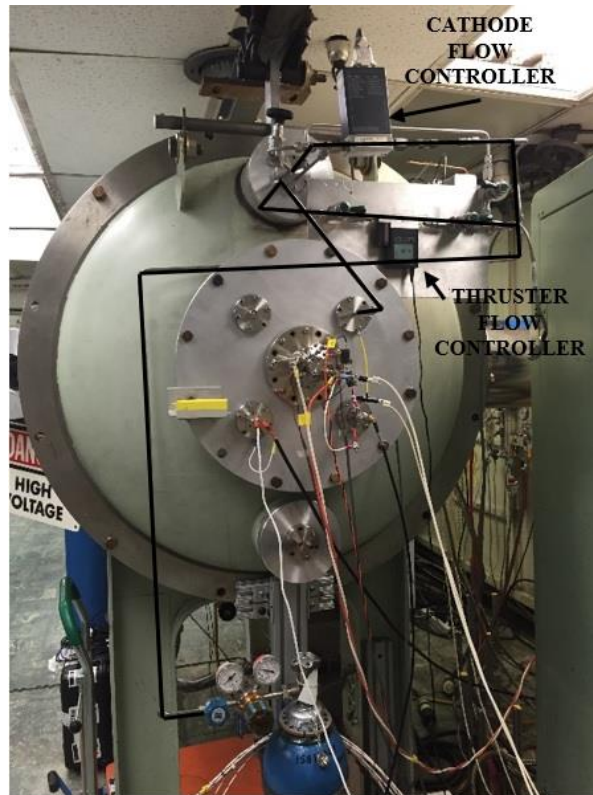
Figure 20: Propellant Feed System used at JPL
